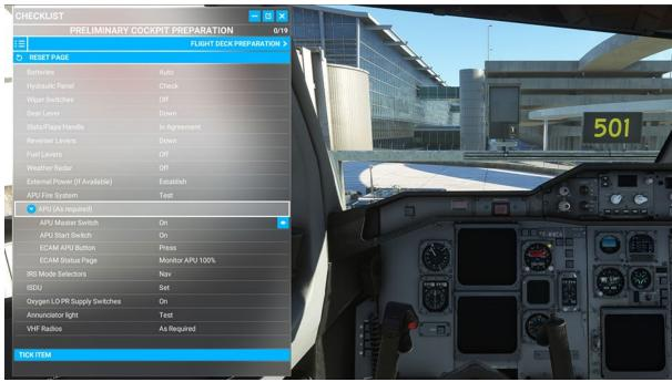
Clicking the blue eye icon to the right of the checklist item will switch your view to the correct panel where the button/switch/dial/gauge is located.
